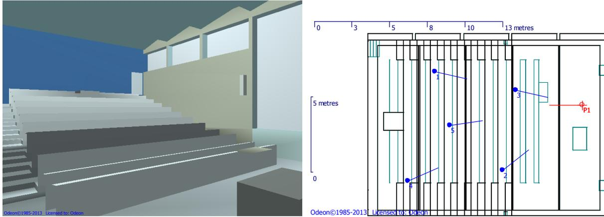
**Figure 5:** Model of the *auditorium 21* at the Technical University of Denmark, as it appears inside ODEON. *Left:* Three-dimensional rendering of Auditorium 21 with colors corresponding to the reflectance of the surfaces<sup>14</sup>. *Right:* Source and receiver positions inside *auditorium 21*.
