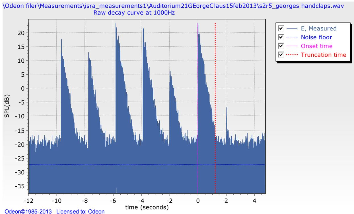
**Figure 3:** Display of onset time and truncation time at 1000 Hz for a series of handclaps. The recording contains multiple impulse responses – ODEON chooses the one with the maximum broad band peak level.
