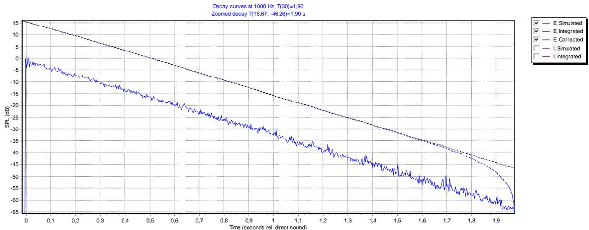
**Figure 1:** Example of simulated squared impulse response curves and integrated decay curves.
