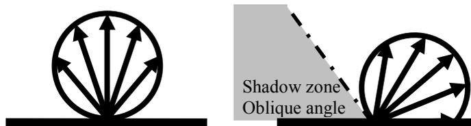
Figure 5: Traditional Lambert directivity to the left and Oblique Lambert to the right. Oblique Lambert produces a shadow zone where no sound is reflected. The shadow zone is small if scattering is high or if the incident direction is nearly perpendicular to the wall. On the other hand if scattering is low and the incident direction is oblique then the shadow zone becomes large.
