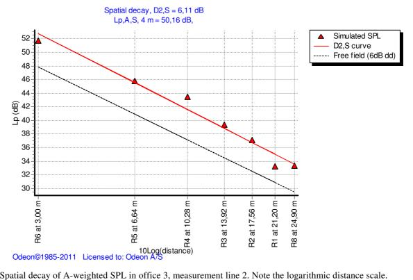
Figure 2. Spatial decay of A-weighted SPL in office 3, measurement line 2. Note the logarithmic distance scale.
