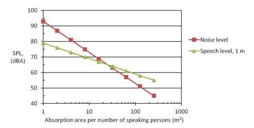
Figure 1: Ambient noise level and assumed speech level as functions of the absorption area per speaking person.
