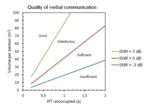
Figure 2: The minimum volume per person required for a certain quality of verbal communication as a function of the reverberation time in unoccupied state. A group size of 3.5 is assumed.
